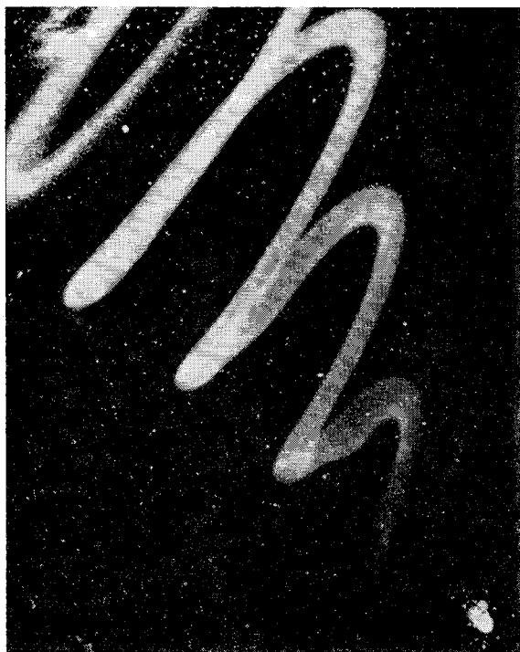
Fig. 13 Photomicrograph obtained as in Fig. 12. Helical trace of small oxide particles formed after development of vapor-phase burning 55
